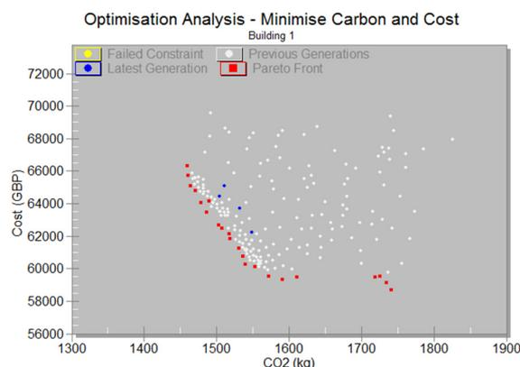
Figure 7: Results obtained from simulating a basic box model. The red points represent a convex Pareto front (Adapted from Huws and Jankovic, 2014).
