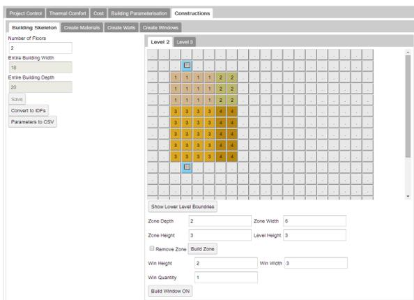
Figure 5: Basic & functional graphical interface of the expert system. It shows the basic 2D representation of the building skeleton, created to represent the floor plan in Figure 4. This is subsequently converted into a 3D physical representation that consists of a complete set of building components.
