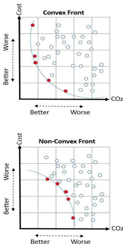
Figure 6: Illustrates the two typical types of Pareto fronts: convex and non-convex.
